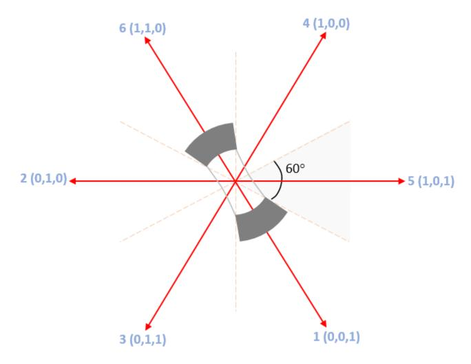
The block uses a commutation logic based on the Hall sequence to generate switching sequences.
