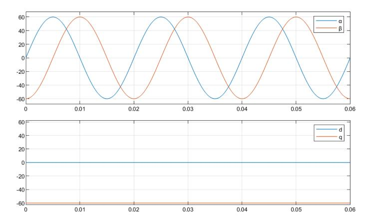
• The q-axis aligns with the  $\alpha$ -axis.
