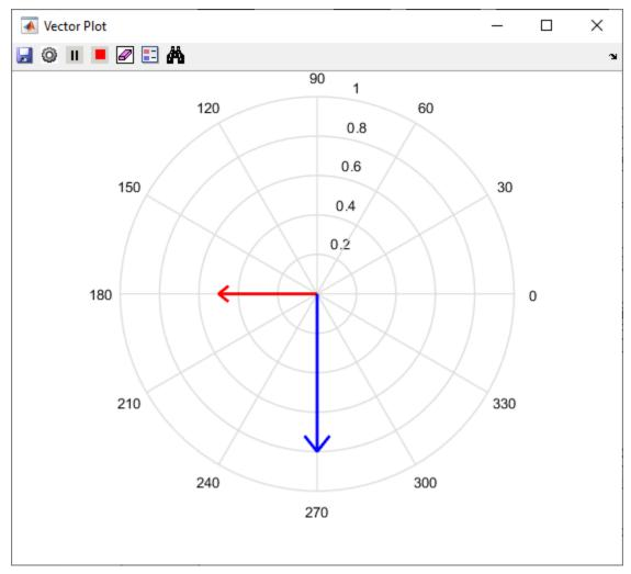
• Stationary Reference Frame — Select this option to plot the three-phase voltage and current vectors in the stationary  $\alpha\beta$  reference frame.
