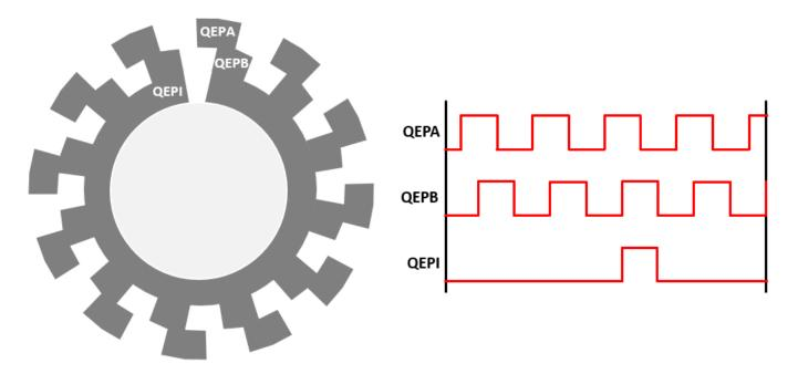
In this example, the timer driven by the QEP increments by four for each slit:
