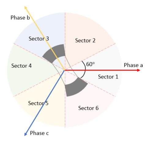
The block uses a commutation logic based on the position sensor signals to generate switching sequences.
