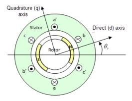
The motor magnetic field due to the permanent magnets creates a sinusoidal rate of change of flux with motor angle.
