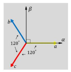
• This figure shows the equivalent  $\alpha$  and  $\beta$  components in the stationary  $\alpha\beta$  reference frame.
